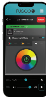
Set Master LED Light Mode and Brightness
